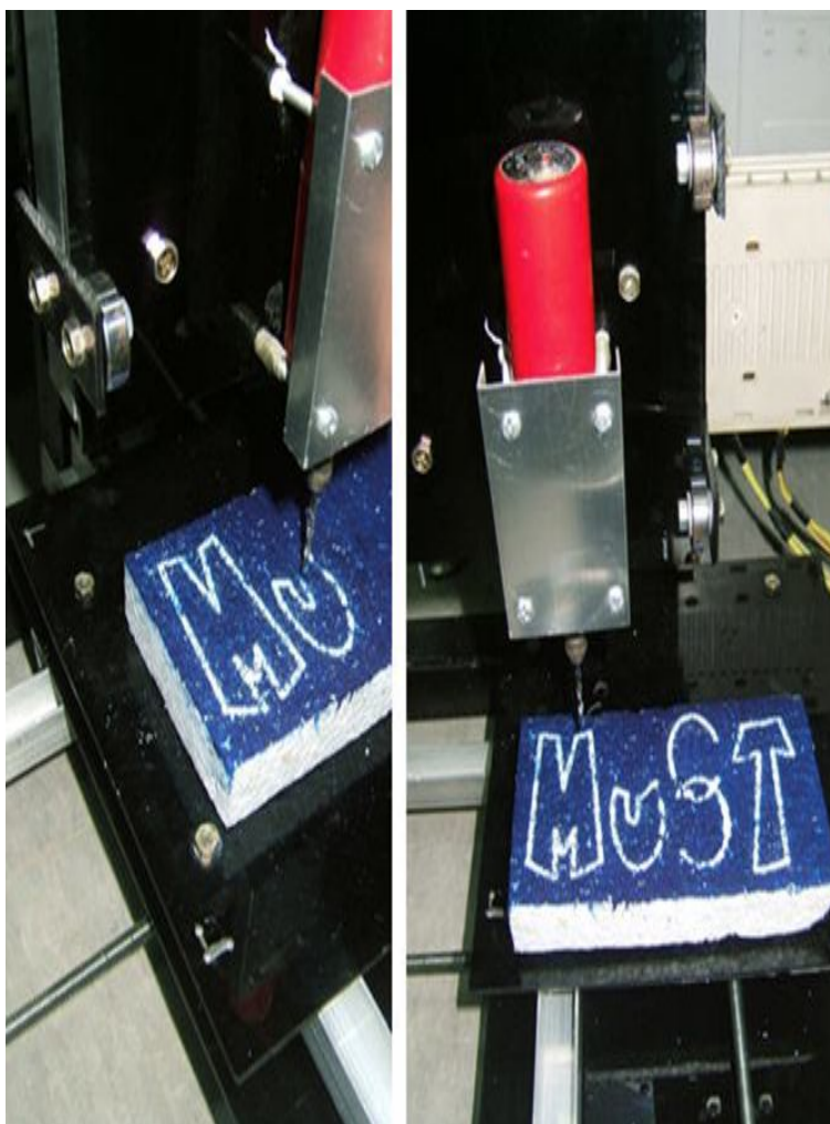
Figure 20: The milling operation
