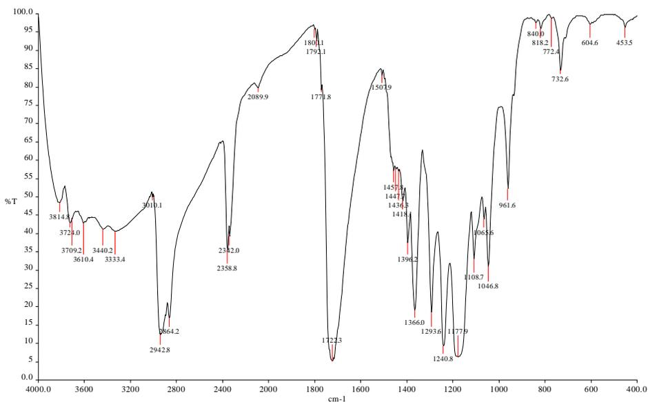
Fig. 2C FTIR spectra of chlorogenic acid loaded polycaprolactone nanofibers
