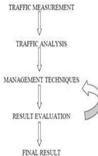
Fig. 1 General Process for Traffic Management
