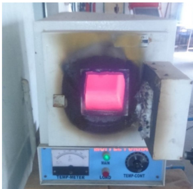
Figure 1 Muffle furnace at 550 0 C
