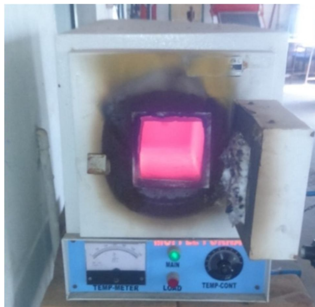
Figure 1 Muffle furnace at 550^\circ\text{C}
