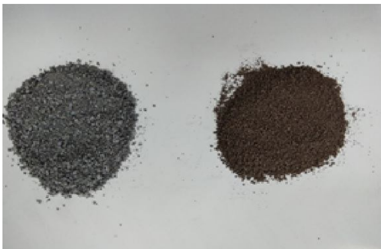
Fig 1: Crushed recycled slag and fresh flux
