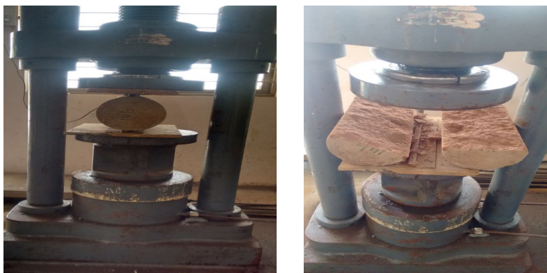
Figure 15 Split tensile strength of CSRE specimens
