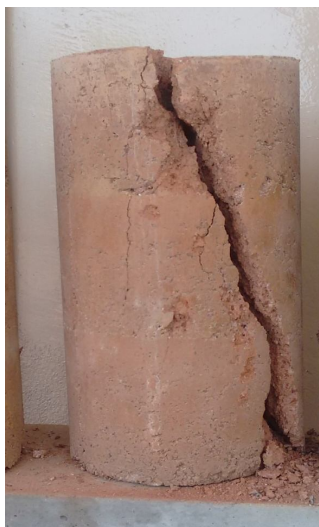
Figure 11 Compressive strength of CSRE specimens
