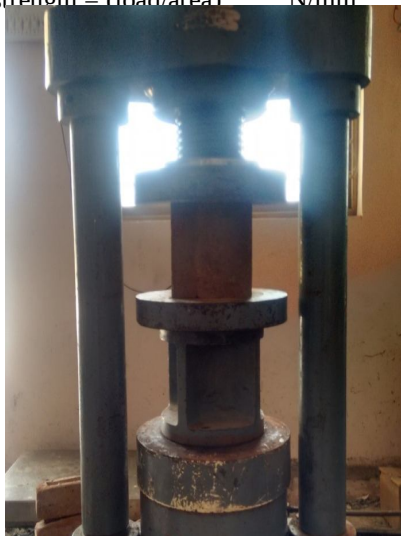
Figure 11 Compressive strength of CSRE specimens
