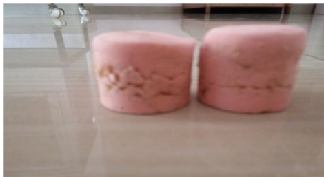
Fig.3 Composite after compressive test
